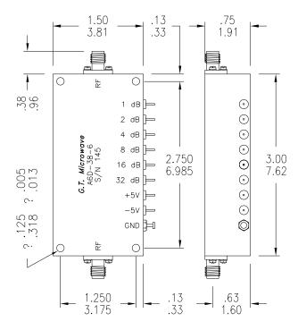
DIMENSIONS ARE EXPRESSED  $_{\text{CM}}^{\text{IN}}$  TOLERANCES ?  $_{.05}^{.02}$  ?  $_{.025}^{.010}$
